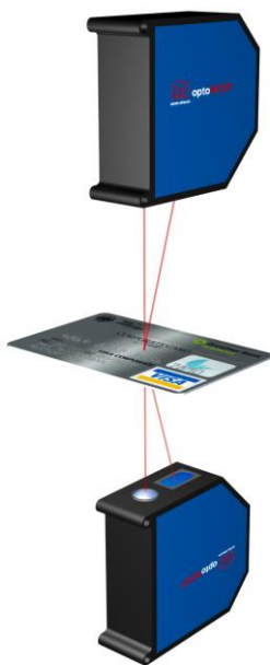
Measurement of thickness and warpage of credit cards
