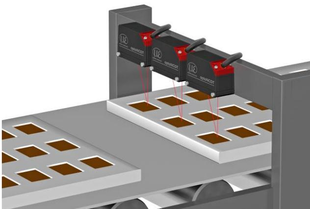
*Thickness measurement of confectionary, mounted as O-frame*
