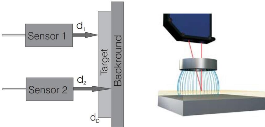
Two sensors are placed at the same distance  $d_1$  from the measuring object on one side of the target. One sensor measures the distance  $d_2$  to the background which is on the opposite side of the object. The thickness  $d_D$  of the target is calculated by subtracting the signals from one another.
