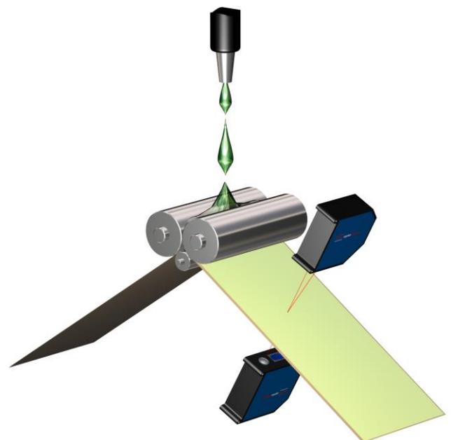
*Thickness measurement of medical plasters*
