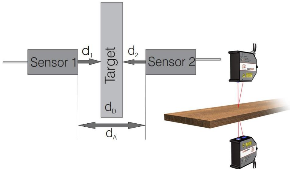
Two sensors are placed at a known distance  $d_A$  on both sides of the measuring object (= target) which each measure the distance to the object. The distances  $d_1$  and  $d_2$  are subtracted from the sensor distance  $d_A$  in order to determine the thickness  $d_D$  of the target.
