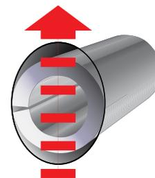
Direction of impact load and resulting hole elongation (*enlargement*)
