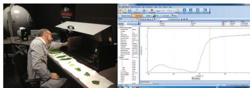
Figure 2 – Using a spectrophotometer and modified goniometer in the Avnet LightLab, I measured the spectral characteristics of various leaf samples.
