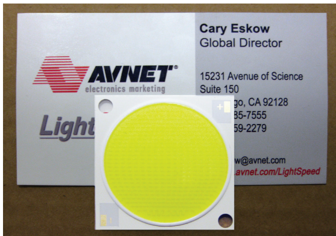
Figure 1—A large CoB LED from Citizen Electronics, available from Avnet
