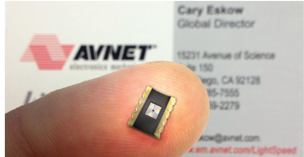
Figure 1 – A precision 6-channel multispectral sensor IC resting on my fingertip
